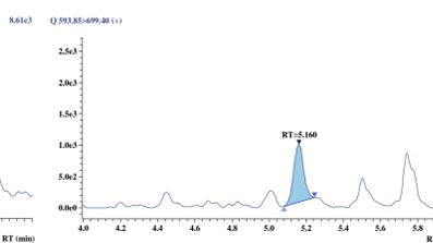
Figure 5. Representative MRM chromatogram of 0.29 µg/mL of cetuximab in Wistar rat plasma
