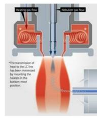
Figure 3. Heated ESI probe
