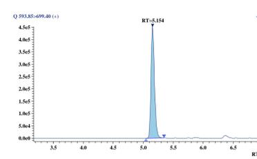
Figure 6. Representative MRM chromatogram of 150 µg/mL of cetuximab in Wistar rat plasma
