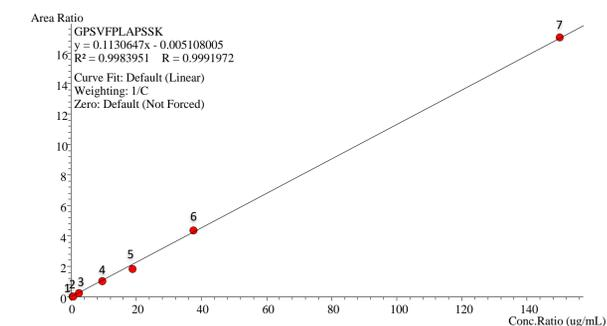
Figure 7. Calibration graph for cetuximab analysis in rat plasma
