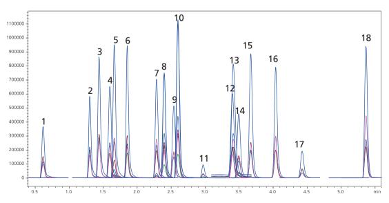
Figure 1. Representative chromatogram of sulfonamide drugs. Standard mixture at 125 pg on-column for each standard. Peak numbers follow the order described for SA compounds in table 1A.
