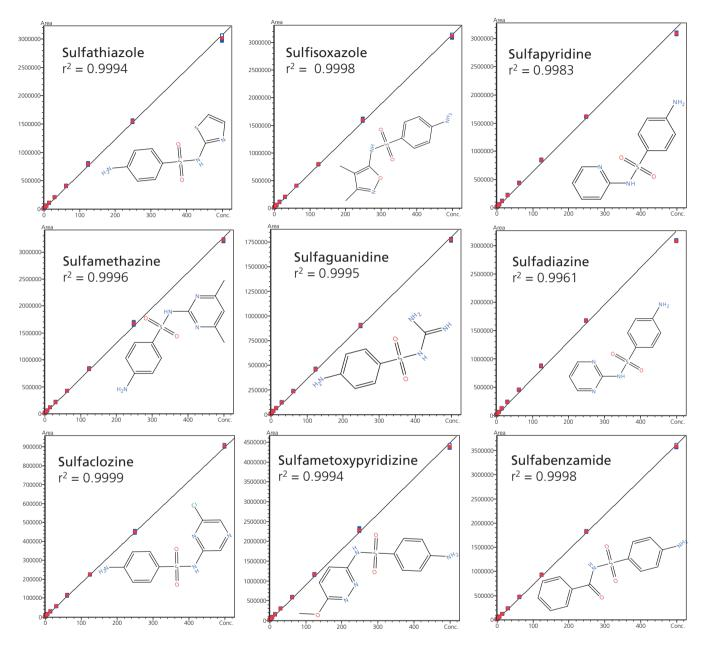
Figure 2. High degree of linearity was observed over the concentration range 0.5–500 pg on column, with values of  $r^2 \ge 0.990$  for all analytes.
