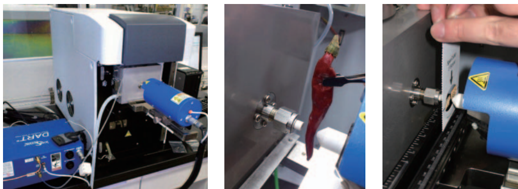
Fig. 1 DART-SVP ion source LCMS-2020
