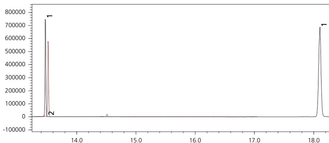
Figure 1 MRM chromatogram of organic tin pesticide derivatives (1.0 mg/L each)
