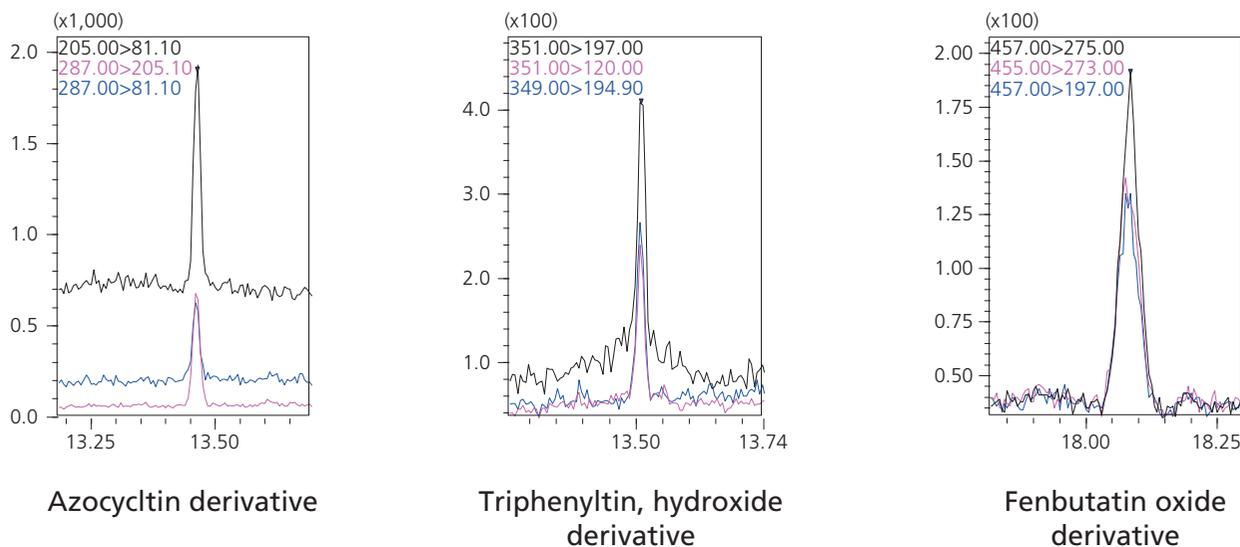
Fig.3. The mass chromatogram of the organic tin pesticide derivatives (1 µg/L each)
