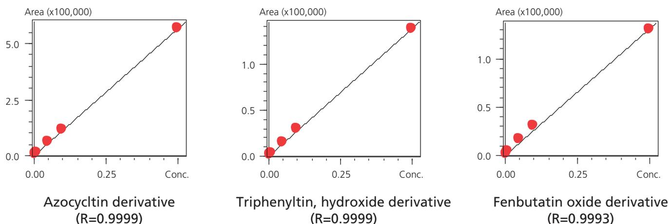
Fig.2. The calibration curve of organic tin pesticide derivatives
