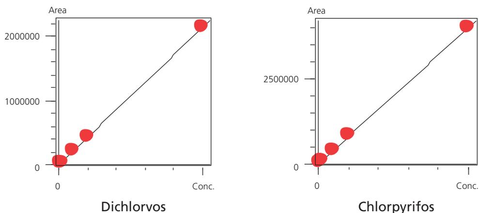
Figure 3. Calibration curve of dichlorvos and chlorpyrifos
