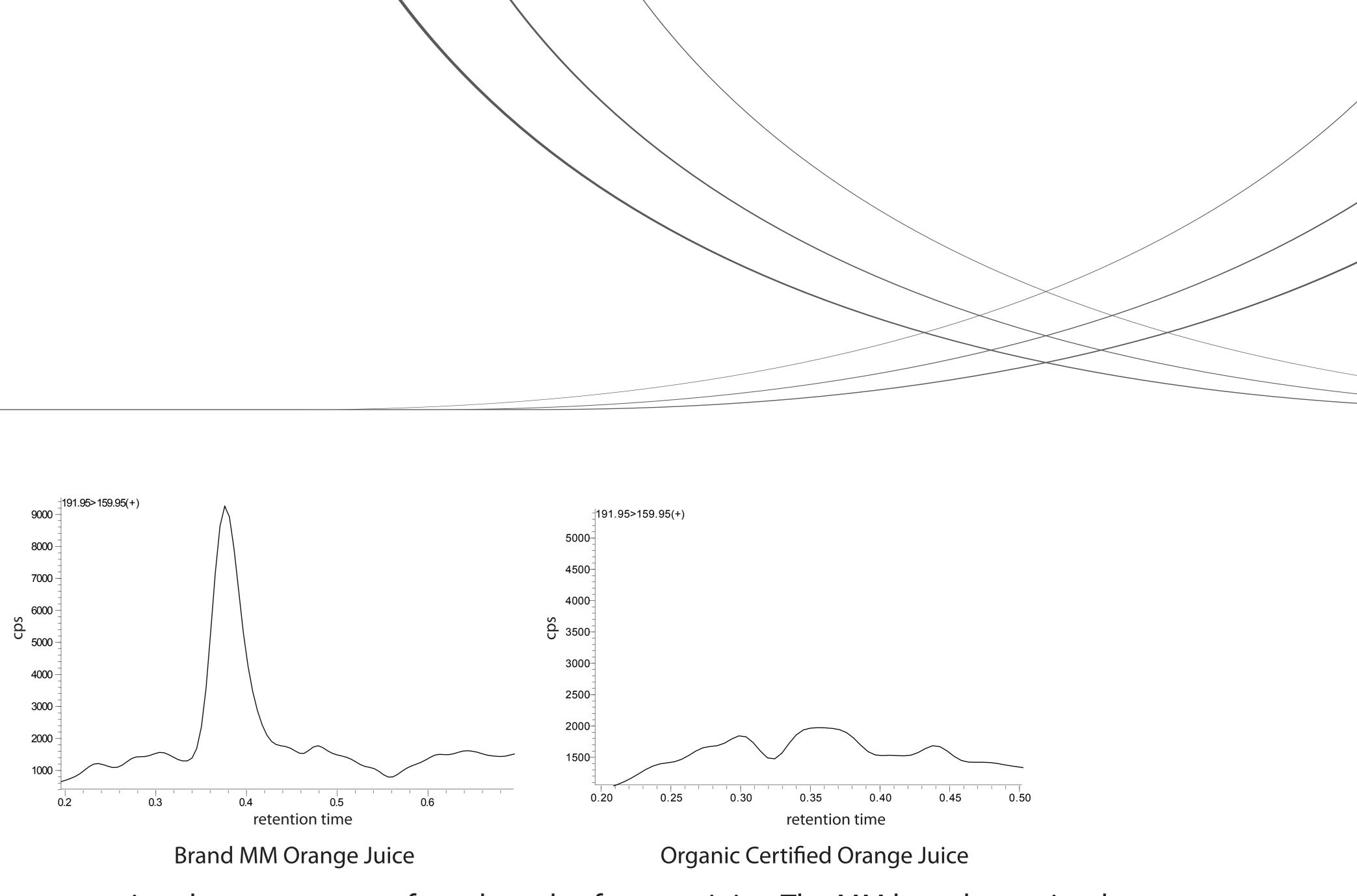
The Nexera UHPLC pumps enabled a fast gradient with a runtime of under 1 minute, while the SIL-30ACMP autosampler enabled injection cycle times of just 7 seconds. The improved ion optics of the LCMS-8040 made it possible to achieve better sensitivity with dilute-and-shoot sample preparation. Not only were the runs rapid, but the retention times and peak areas were extremely reproducible as well, with relative standard deviations of just 0.55 and 2.98% respectively.
