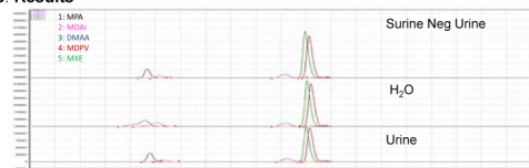
Figure 1. Total Ion Chromatogram of selected transitions obtained from the analysis of 1,000 ng/mL standard mix in three different matrices.
