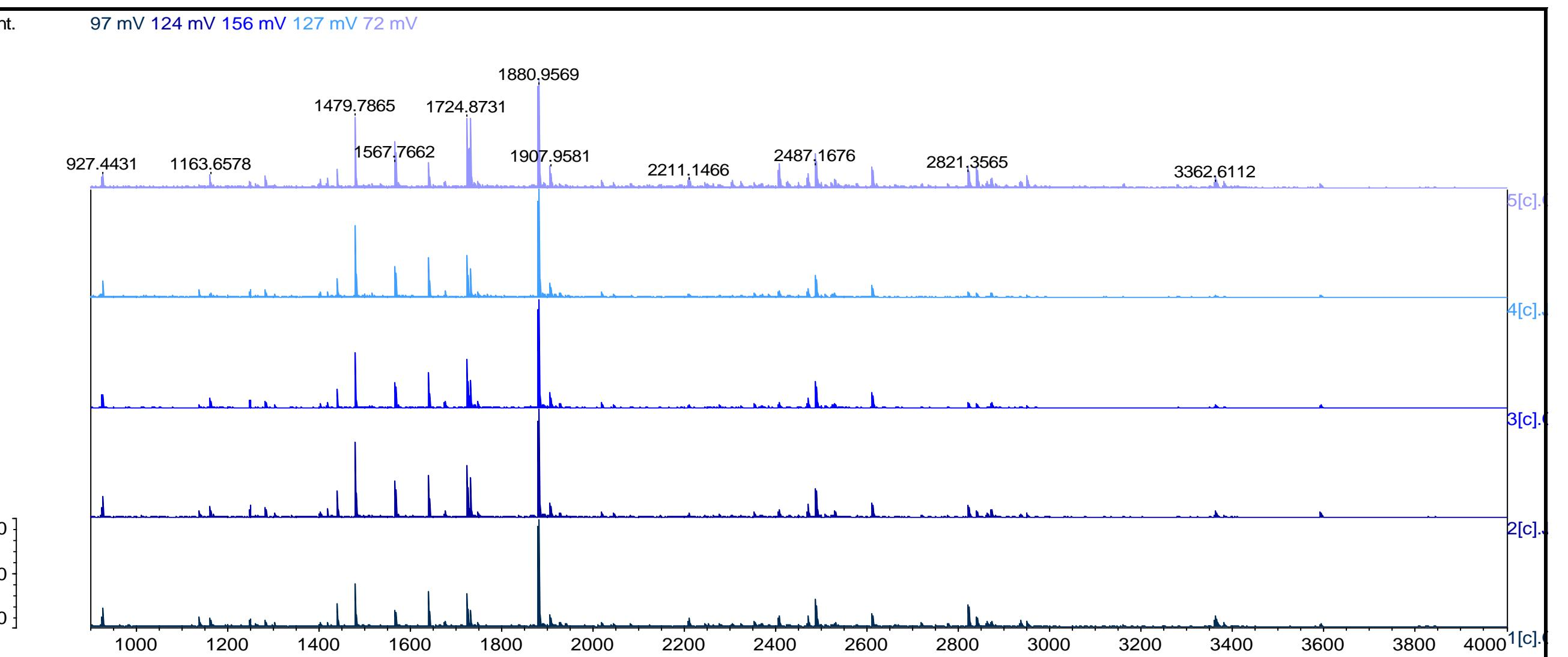
**Reproducibility Assessment:** Peptide Mass Fingerprints from five injections of myoglobin (B) and albumin (C). Comparison of the features in the spectra indicate that the workflow of the modified Perfinity Workstation using the enhanced immobilized trypsin IMER column provides excellent reproducibility for the peptide mass finger print workflow with a six minute digestion time.
