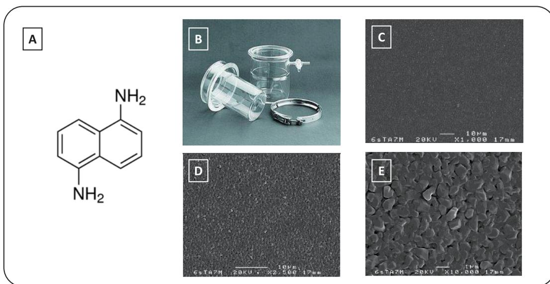
Figure 1 Structure of 1,5- Diaminonaphthalene (1,5-DAN) (A), the Ace Glass Sublimation glassware (B) and SEM images of the DAN crystals (matrix density of  $89 \mu\text{g}/\text{cm}^2$ ) at x1,000 (C), x2,500 (D) and x10,000 (E) magnifications. The homogenous matrix deposition of 1,5-DAN via sublimation can be seen in the SEM images with an average crystal size of  $\sim 3 \mu\text{m}$
