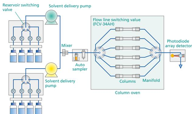
Fig. 2 Flow Line Diagram of Nexera Method Scouting System (Shown with Six Types of Columns)
