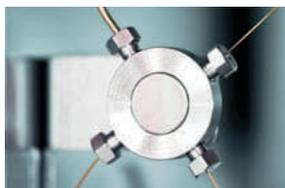
Sample loss is reduced with a deactivated splitting device.
