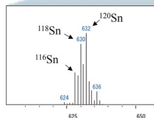
Components that are thermally degradable or difficult to vaporize are not suited to GC analysis. Their mass spectra can be obtained easily using the DI probe. Above is an example of Sn-phthalocyanine spectra obtained using the DI Probe.
