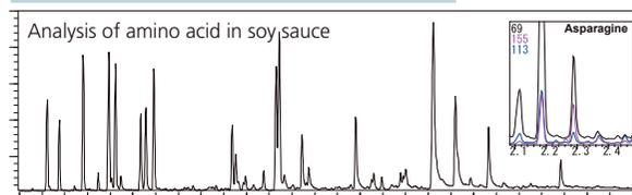
This database consists of a mass spectra library (with retention indices) for amino acids, fatty acids, and organic acids and method files in which analytical conditions and data analysis conditions for the analysis of amino acids, fatty acids, and organic acids are set.
