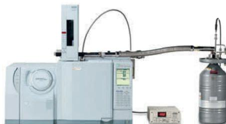
The Comprehensive GC/MS (GC×GCMSq) technique employs a modulator to link two capillary columns of complementary orthogonal phases. The technique requires a GC-MS system capable of very fast data collection to fully capture the very narrow, fast eluting compounds. Sensitivity is also an important requirement for many Comprehensive GC×GC applications.
