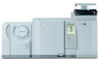
Thermal Desorption is a technique for air sample concentration. It utilizes a small tube filled with the appropriate sorbent material. Samples are collected in the field and transported.
