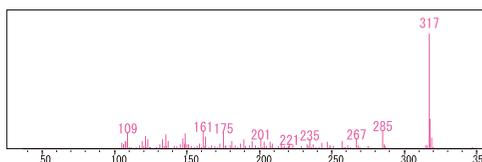
Mass spectrum of cis-5,8,11,14,17-Eicosapentaenoic Acid Methyl Ester (C<sub>20</sub>:5n<sub>3</sub>) in EI and CI
