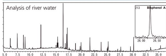
Simultaneous GC/MS analysis supporting identification and quantification of 942 environmental pollutants can be performed. The retention times and calibration curve information of environmentally hazardous chemical substances are registered, so approximate concentrations can be obtained with compounds even when it is difficult to obtain standards.
