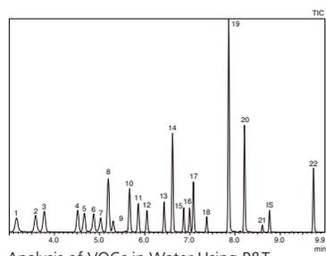
The combination of a high-speed GC/MS method and a fast oven cooling rate dramatically reduces the analysis cycle. This VOC analysis is reduced by more than half.
