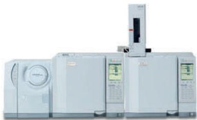
A multi-dimensional GC/GCMS system performs separation using two columns of orthogonal phases. The system employs a pressure switching heart-cut device (Multi-Deans Switch) to direct the effluent of the first column on to a second column. The Multi-Deans Switch assembly has been designed to install directly into a GC-2010 Plus and be combined with a GCMS-QP2010 Ultra. This system provides the ultimate in chromatographic performance.
