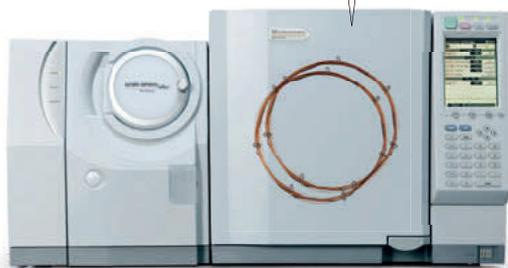
Installing two columns in one MS is possible with the GCMS-QP2010 Ultra because of its high-capacity dual-inlet turbomolecular pump.
