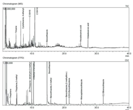
Simultaneous detection using MS and FPD of a pyrolyzed rubber sample
