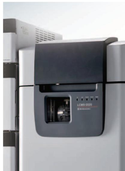
High-Throughput Liquid Chromatograph Mass Spectrometer
