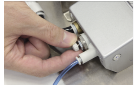
Grip force is changeable by air pressure adjusting screw
