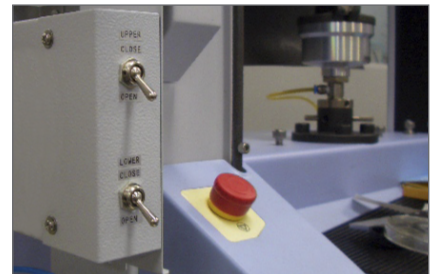
Grip force is changeable by air pressure adjusting screw
