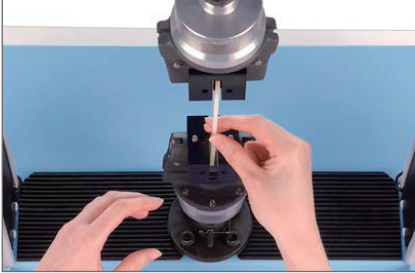
The foot valve unit frees both hands to mount specimens
