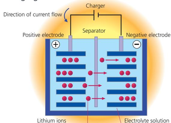
Lithium ions in the lithium compound (positive electrode material) pass through the separator and into the layers in the carbon negative electrode material, resulting in a charging current flow.
