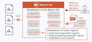
i-QLinks seamlessly links sample information and analysis conditions to analytical instruments for efficient testing. Data acquired from an analytical instrument is automatically transferred to a pre-configured spreadsheet template for creating test reports. This reduces the risk of falsification and human error, enabling highly reliable testing.
