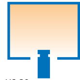
HS-20 Conveyance from the bottom makes it difficult for heat to escape from inside, improving oven temperature stability. (Patent pending)
