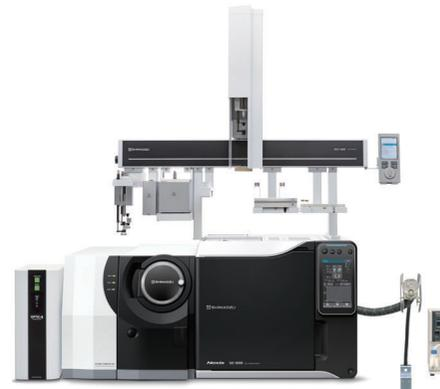
Since some odor components have a low odor threshold, low concentration levels need to be detected to identify the causative substances. High-sensitivity MRM/SIM analysis by GC-MS/MS can reliably detect even trace components near the odor threshold (a few pg/g).
