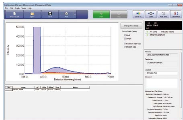
Fluorescence Quantum Efficiency Measurement Window (Fluorescence quantum efficiency measurement of quinine sulfate)
