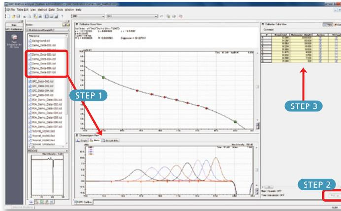
**STEP 1** Drag and drop standard-sample data into the window.
