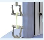
Tensile and Shearing Test for Noodles
