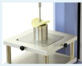
Potato Chip Breakage Test
