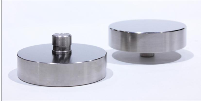
Fixed compression plates, or platens as they are otherwise known, are versatile testing accessories, applicable to compression and cycle testing a diverse range of materials and finished products. Hardened faces, surface hardness of 60 on the Rockwell HRC scale, ensure minimal wear, preserving surface smoothness.
