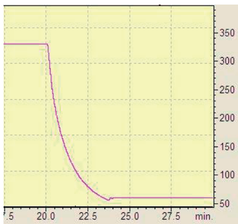
Figure 1: GC oven cooldown from 330°C to 60°C in 4 minutes
