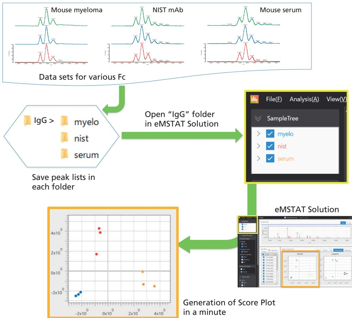
Fig.6 Classification of three Fc using eMSTAT Solution
