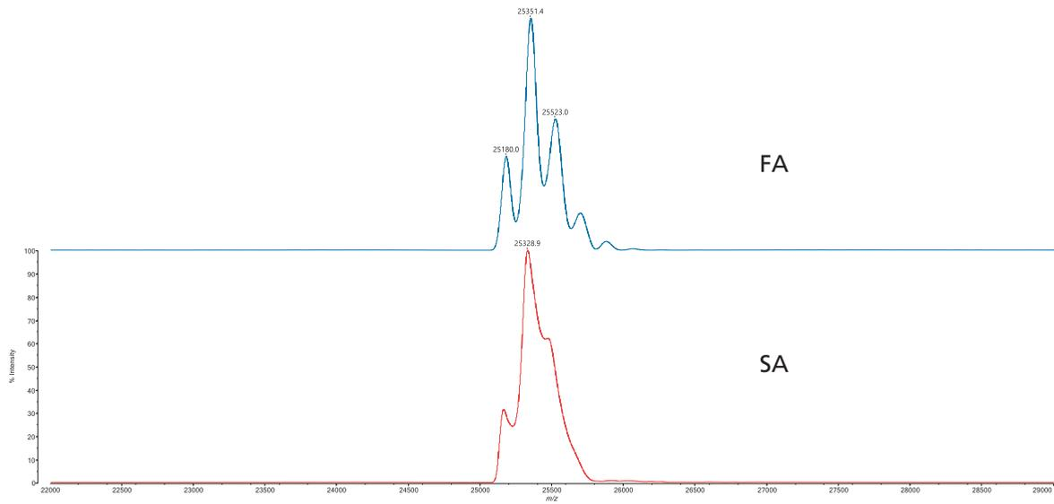
Fig.4 A comparison of Fc measured with SA and FA under the identical MS condition
