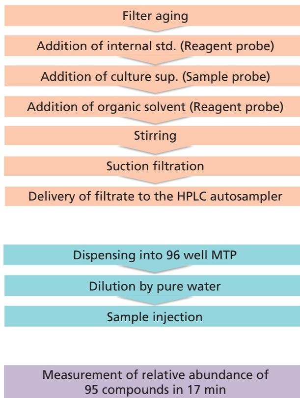
Fig.2 Pretreatment and measurement flow
