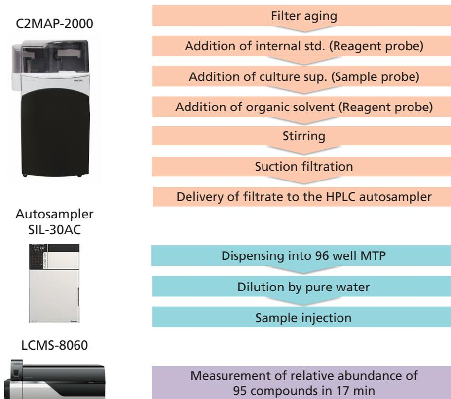
Fig.2 Pretreatment and measurement flow
