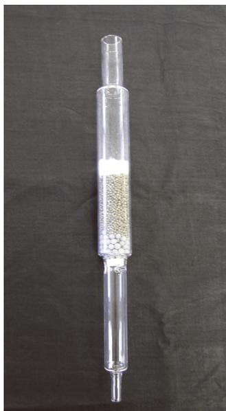
Fig. 1 High-Salt Sample Combustion Tube
