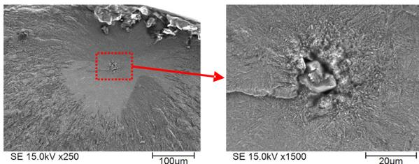
**Fig. 2 Observation Image of an Inclusion in Specimen #1 (Secondary Electron Image)**
