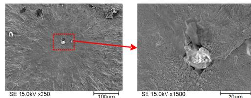
Fig. 7 Observation Image of an Inclusion in Specimen #3 (Secondary Electron Image)
