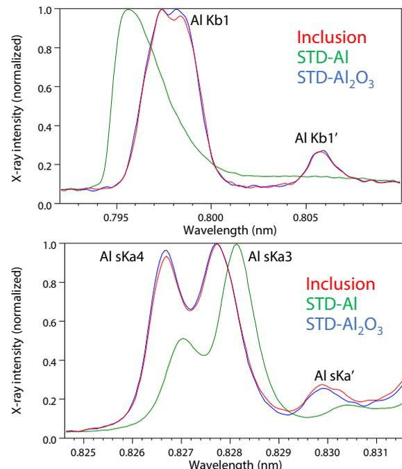
**Fig. 4 Al State Analysis (Upper: Al Kb Lines, Lower: Al sKa Lines)**
