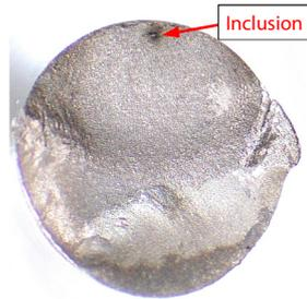
**Fig. 1 Photo of the Fractured Surface (Optical Microscope)**
