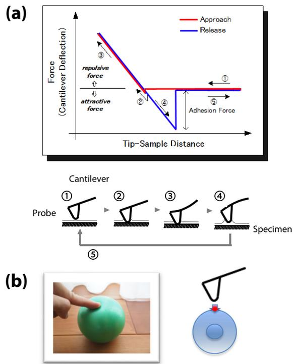
Fig. 5 Explanation of Force Curve Measurement
