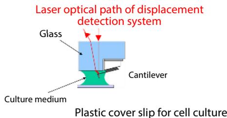
Fig. 4 Configuration of Observation in Solution
