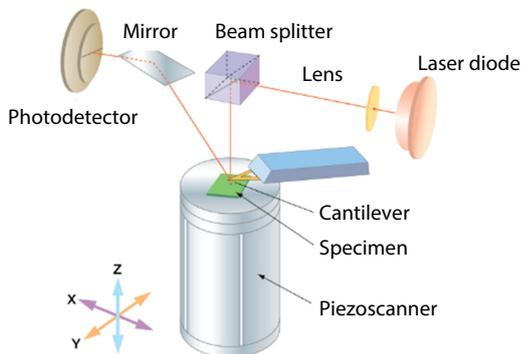
Fig. 3 Configuration of SPM
