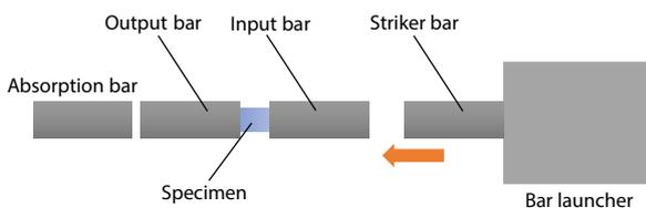
**Fig. 1 Schematic Diagram of the Hopkinson Bar Method**
