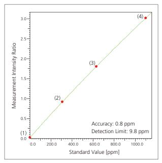
Fig. 2 Calibration Curve for Sb in Plastics
