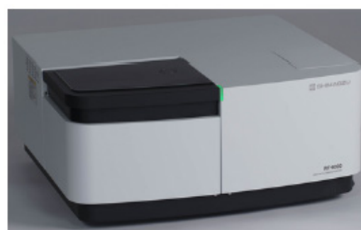
Fig. 1 Shimadzu spectrofluorophotometer, RF-6000, used for fluorescence measurements
