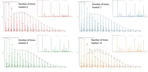
Fig. 3 Mass Spectrum of General-purpose Polyester after Dissolution/Reprecipitation Treatment
