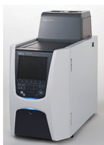
Fig. 6 TOC-L Total Organic Carbon Analyzer + TNM-L Total Nitrogen Unit
