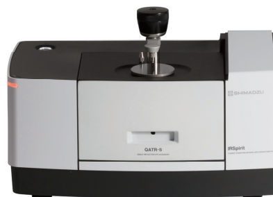
Fig. 1 QATR-S Accessory Installed in IRSpirit Sample Compartment
