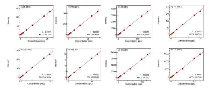
Fig 2. Calibration curves obtained in present study
