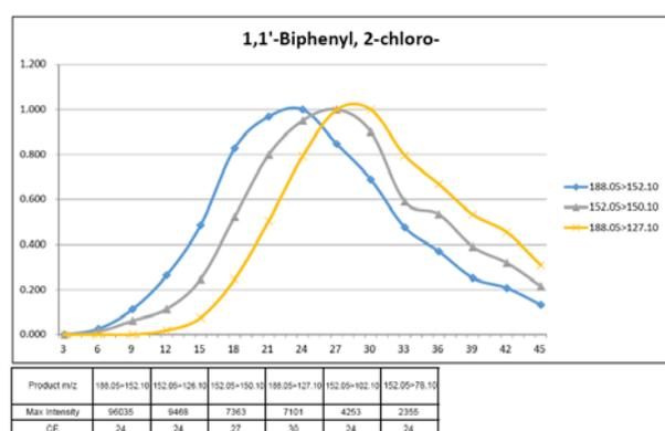
**Figure 1. CE Optimization using Smart MRM optimization tool**
