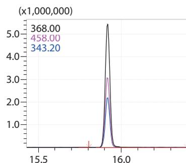
Fig. 4 Mass Chromatogram of 8 µg Sample of Cholic Acid
