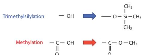
**Fig. 2 Schematic Diagram of Derivatization with Trimethylsilylation of Hydroxy Groups, Methylation of Carboxyl Group.**
