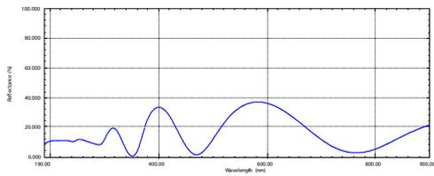
Fig. 6 Spectrum of 0.4  $\mu\text{m}$  Resist Film
