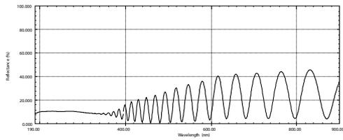
Fig. 4 Spectrum of 3.0  $\mu\text{m}$  Resist Film
