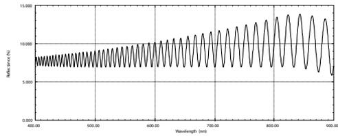
Fig. 8 Spectrum of 10  $\mu\text{m}$  Film
