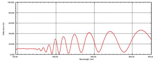
Fig. 5 Spectrum of 1.1  $\mu\text{m}$  Resist Film
