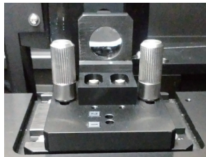
Fig. 4 Micro Beam Lens Unit
