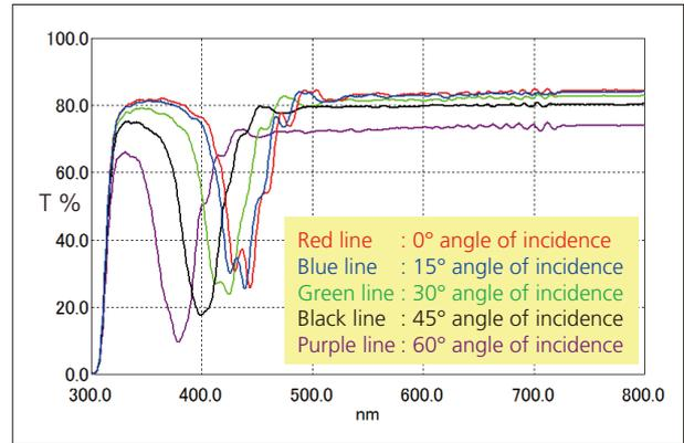
Fig. 5 MLF-13.0 Film Transmission Spectra
