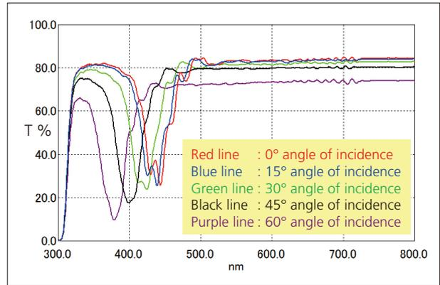
Fig. 5 MLF-13.0 Film Transmission Spectra
