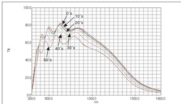
Fig. 4 Transmittance Spectra Measured with s Polarized Light at 0, 10, 20, 30, 40, and 50 Degrees
