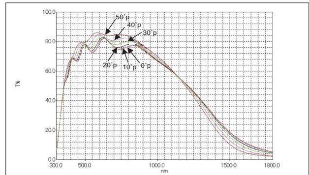
Fig. 5 Transmittance Spectra Measured with p Polarized Light at 0, 10, 20, 30, 40, and 50 Degrees
