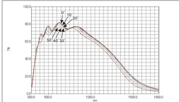
Fig. 6 Transmittance Spectra of Nonpolarized Light Calculated using s Polarized Spectra and p Polarized Spectra at 0, 10, 20, 30, 40, and 50 Degrees
