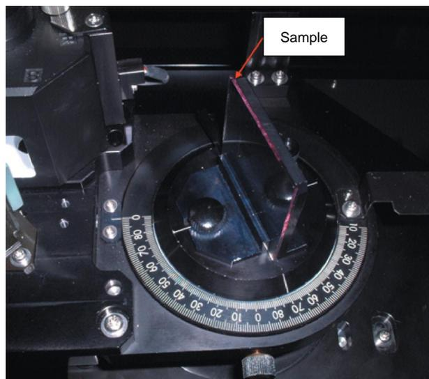
Fig. 2 Sample Mounted on Variable Angle Absolute Reflectance Attachment
