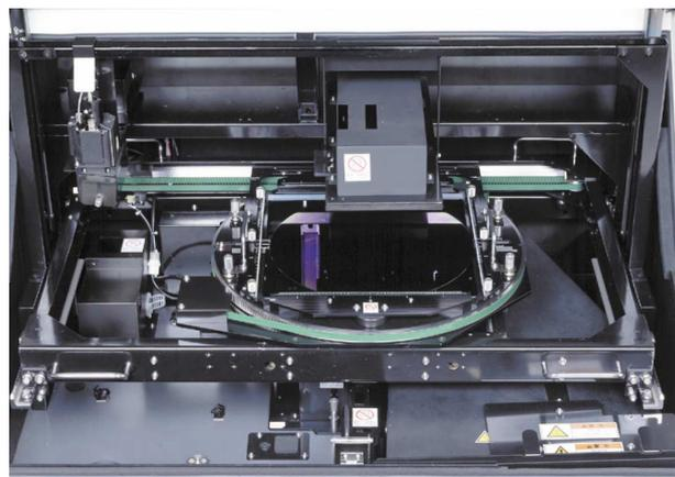
Fig.3 12-inch Wafer Set on Automatic X-Y Stage
