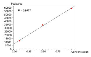
Fig. 7 Calibration Curve of Formic Acid
