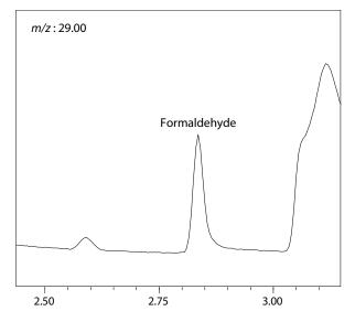
Fig. 4 SIM Chromatogram of 0.1 ppm Formaldehyde Standard Solution
