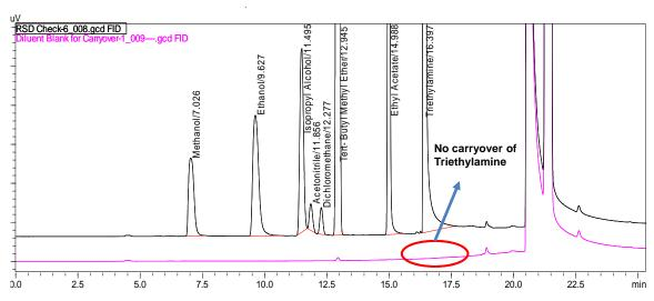
Figure 2: Overlay of Standard solvent mixture and diluent blank on Nexis GC-2030 with HS-20
