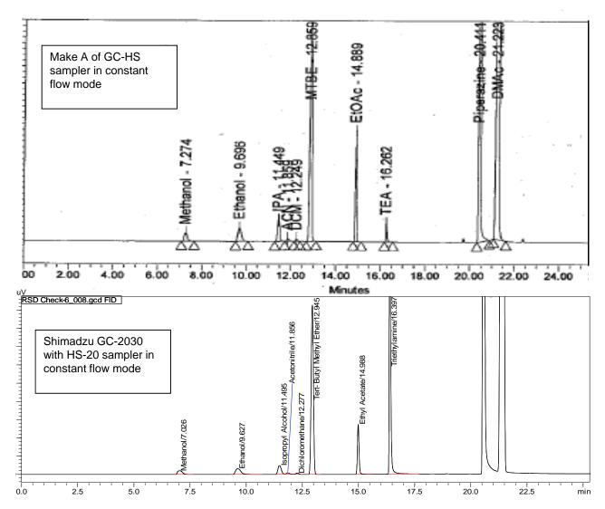
Figure 1: Comparative chromatographic peak profile on Make A of GC-HS and Shimadzu Nexis GC-HS
