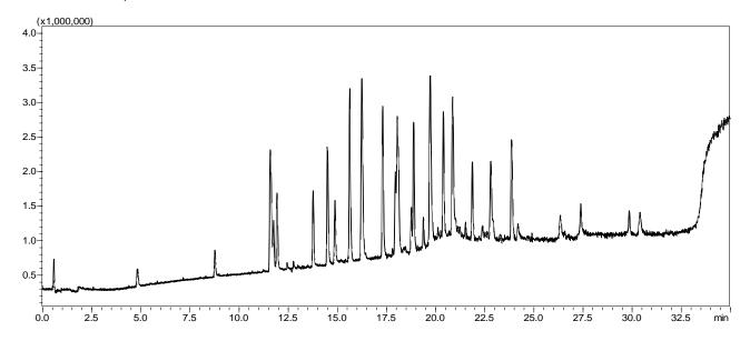
**Figure 1:** TIC in full mass range mode of a mixed standard of 34 PFASs with each at 100 ng/mL in Milli-Q<sup>®</sup> water. Peak ID, RT and mass accuracy are shown in Table 2.
