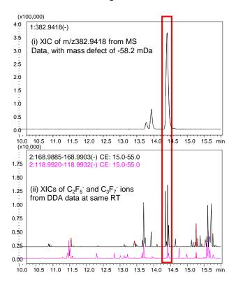
**Figure 5:** Illustration of finding an undiscovered PFAS: (i) XIC of (-)m/z 382.9417 from MS data via mass defect filtering; (ii) XIC of  $C_2F_5^-$  and  $C_3F_7^-$  ions from DDA data, (iii) MS spectrum and formula prediction, (iv) MS/MS spectrum and structural analysis; (v) assignment of fragment ion using Structural Analysis s/w.
