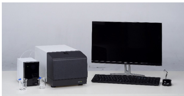
Fig. 1 iSpect™ DIA-10 Dynamic Particle Image Analysis System
