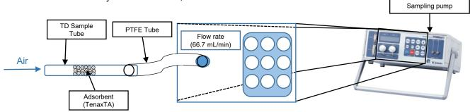
Fig. 1: Sampling pump experimental setup for indoor air sampling
