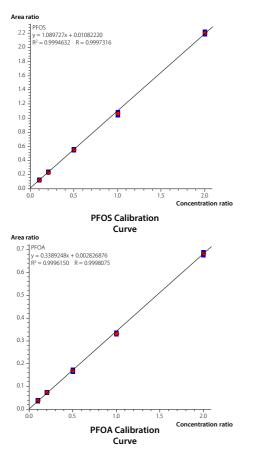
Fig. 3 Calibration Curves of PFOS and PFOA (standard mixture)
