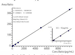
Fig. 2 Calibration Curve (0.5 - 10000 pg/mL)
