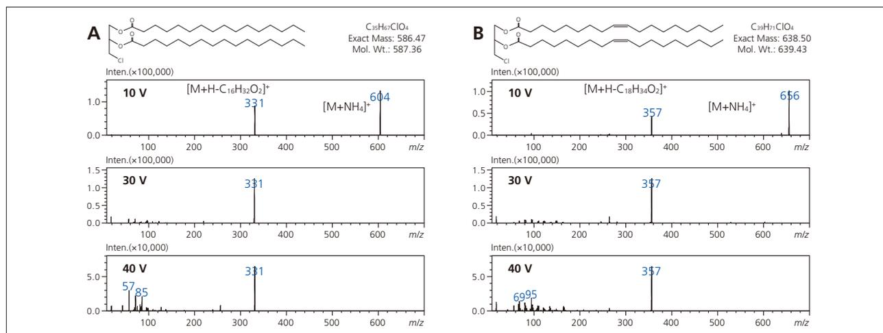
Fig. 1 MS/MS Spectra of the Synthetic Samples (A: 3-MCPD-Dipalmitoyl Ester, B: 3-MCPD-Dioleoyl Ester)
