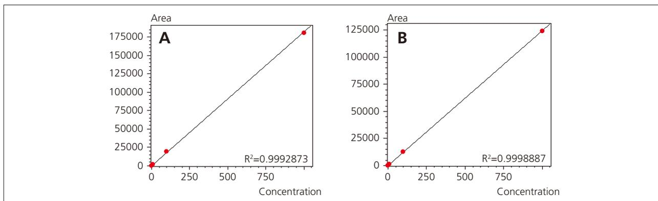
**Fig. 3 Calibration Curves (1–1000 µg/L, n = 6)**
