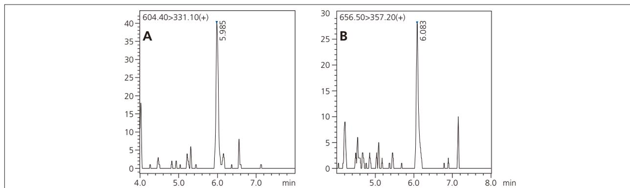
Fig. 2 MRM Chromatograms of the Synthetic Samples (1  $\mu\text{g/L}$ , A: 3-MCPD-Dipalmitoyl Ester, B: 3-MCPD-Dioleoyl Ester)
