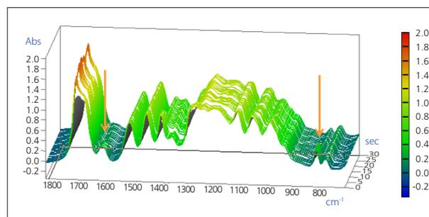
Fig. 3 3D Spectra of Rapid Scan Measurement Generated in Curing Reaction in UV-Irradiated Resin
